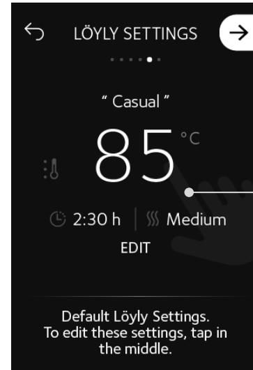
These are the löyly settings for the default profile. Control Panel has three default profiles with preset temperature, sauna time and löyly quality.
