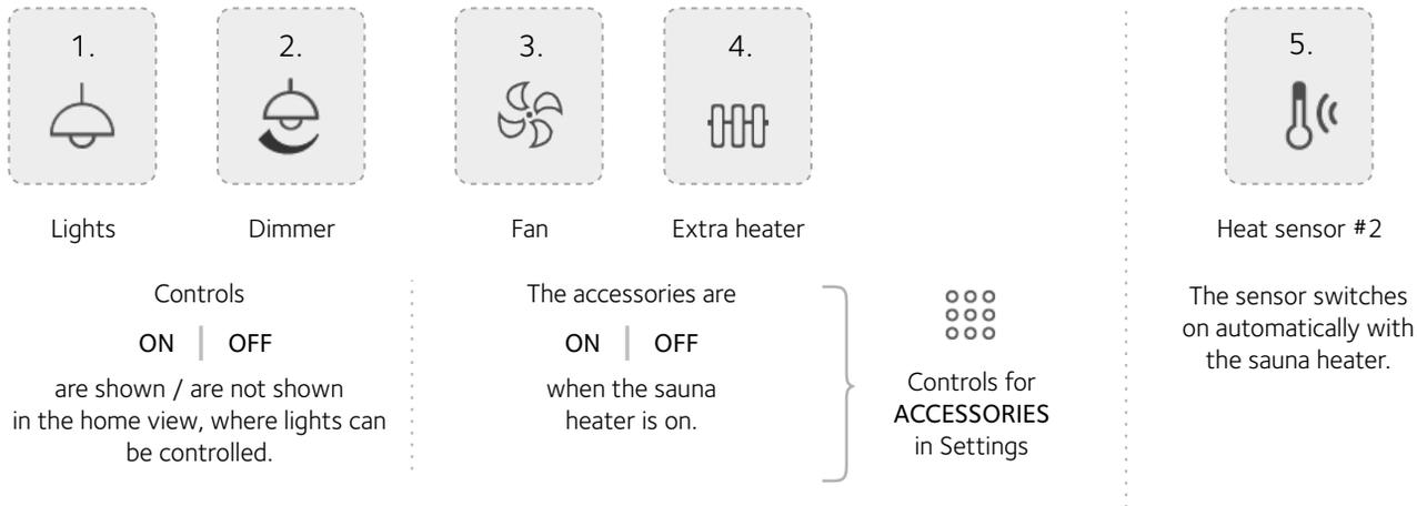
Select physically installed devices that are connected to the sauna heater. You can select the device by tapping on the icon that says "Show". You can deselect it by tapping the "Hide" icon.
