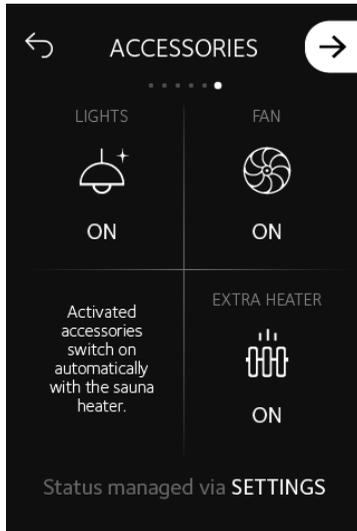
This is a preview of the physically installed accessories, connected to the sauna heater and control panel. All connected accessories are activated automatically, and you can control or monitor them through the control panel settings. Tap the NEXT button and continue to the end of the guide.
