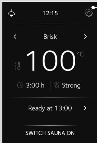
You can access the control panel's settings by tapping the icon (1) in the top-right corner of the screen.
