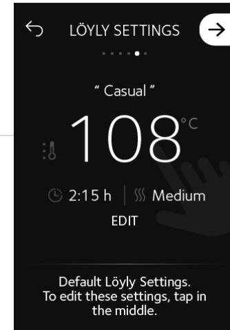
Adjust the profile löyly settings to suit you and tap the OK button at the bottom of the screen.
